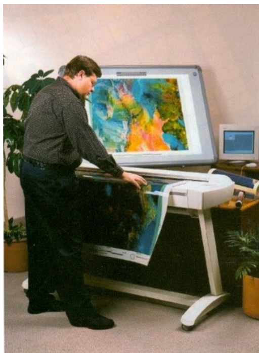
5.15-rasm. A1 formatli kartalarni skanerlovchi qurilma (Manba: Longley, 2005)
