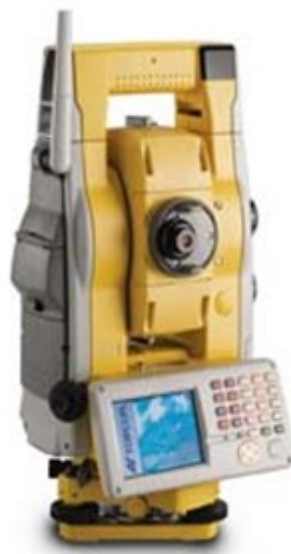
3.10-rasm. Zamonaviy teodolit (Manba: Trimble veb-sahifasi)
