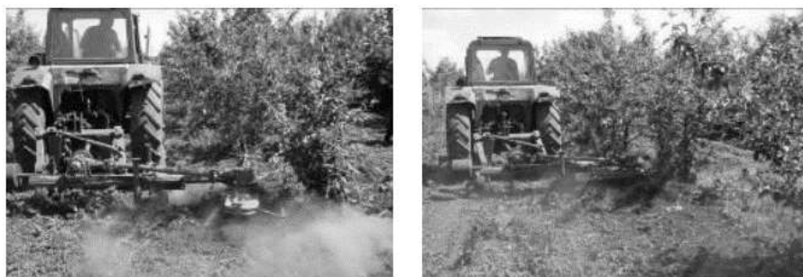
2-rasm. MPP-1.2 bog' frezasining ish jarayoni
