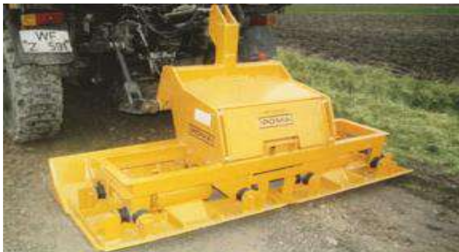
Figure 1. The working space of the compaction machine, which vibrates the soil by vibrating motion
